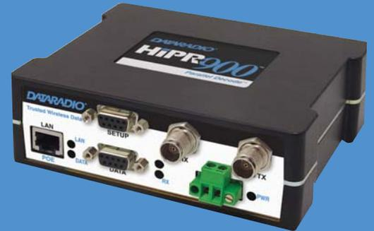
**Dataradio's** new HiPR-900<sup>™</sup> with Dataradio's Parallel Decode<sup>®</sup> technology provides optimal IP communications for reliable, long-range communications in a private wireless data network. With the HiPR-900, you can extend your IP-based network into the field for mobile, SCADA and industrial applications.
